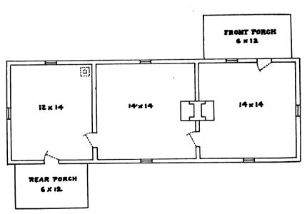
Fig. 30.—PICTURE AND PLAN OF "SHOTGUN" TYPE OF HOUSE COMMON IN SOUTHERN COMPANY TOWNS.
